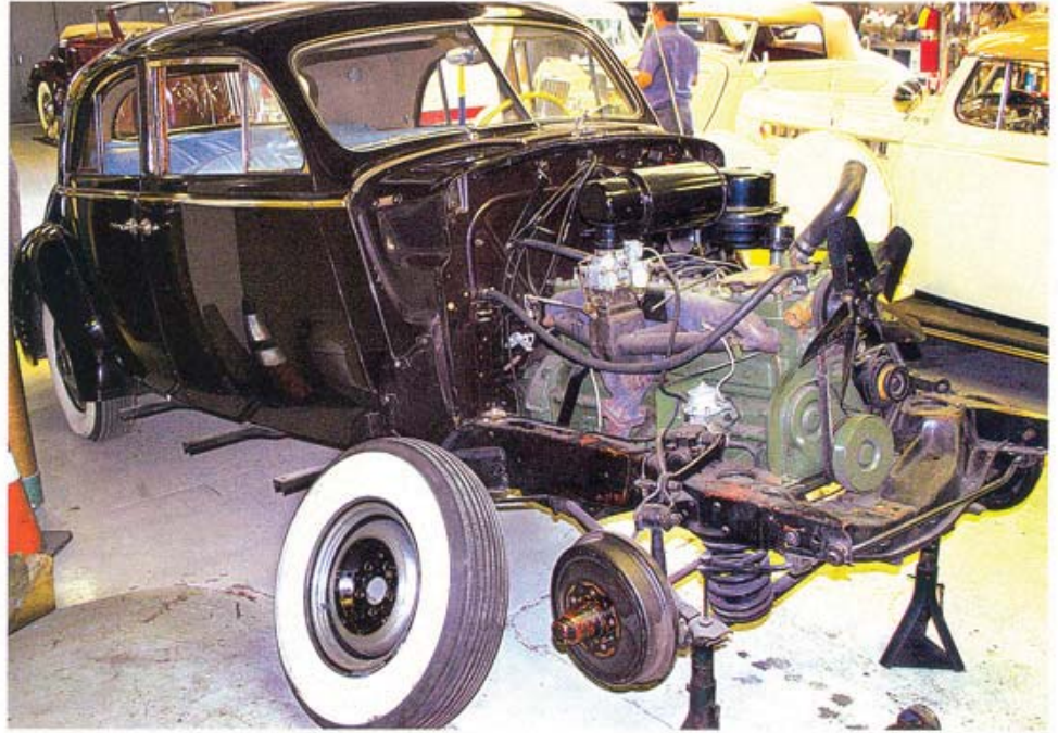
With its prominent grille and front body panels removed, this 1941 LeBaron-bodied Packard is at the initial stage of a complete, body-off, ground-up restoration
