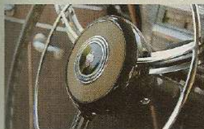
Banjo steering wheel was an option and absorbed the shocks of marginal roads
