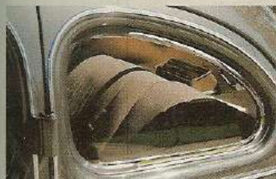
Air conditioning discharge duct is behind the back seat. Vent window is for milder days
