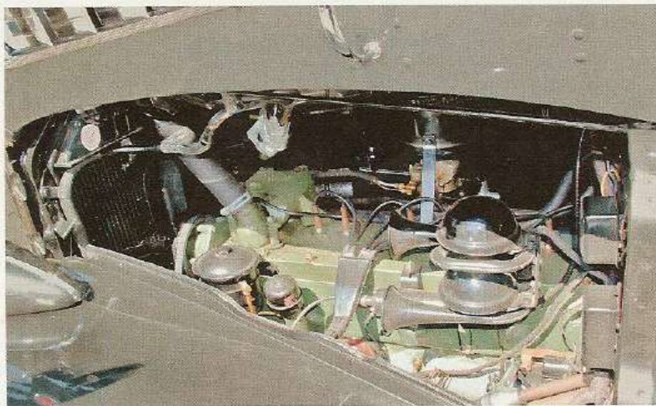
Packard's 282-cu.in. straight eight is velvety smooth and bulletproof. A 245-cu.in. straight six was offered in the 110, and a 356-cu.in. straight eight came in the 160 and 180 models
