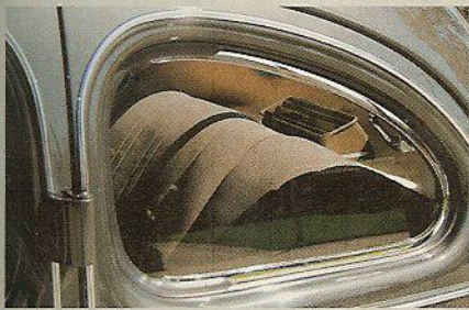
Air conditioning discharge duct is behind the back seat. Vent window is for milder days
